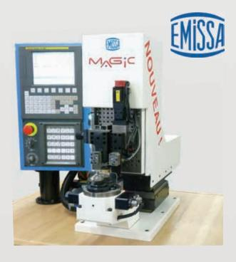
EMISSA compagny has developped a full machining solution for drilling spring bar holes. This smart machine called MAGIC TOOL 50 utilize two PIBOMULTI modules simultaneously to drill **perpendicular** holes between lugs. A turning table allows to load in hidden time. Full documentation is available at EMISSA.
